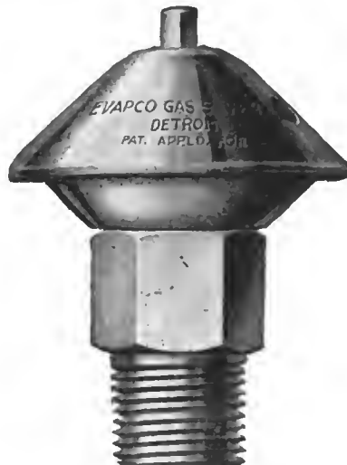
Evapco auxiliary air valve, which automatically feeds additional air to the intake manifold in proportion to the engine speed
